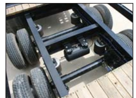
TRAILER FLEX TrailerFlex Air Ride Suspension
